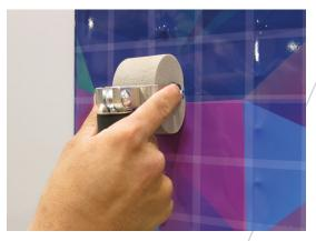
Heat a section of film which covers 4-5 rivets. As you apply heat, the film will wrinkle but will flatten out once it reaches its optimum temperature (180°F to 240°F).
