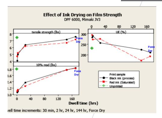
The graph above depicts basic properties of the PVC film itself: tensile strength at break, tensile strength when film is stretched 10% of its original length and elongation at break. The diamond in the upper left shows the properties of unprinted film. As with the previous example of adhesion all printed film characteristics recover, that is the PVC regains strength and body, as it dries.
