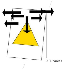
Air is easily trapped between the surfaces of the adhesive and sign surface. A signage installer who keeps an opening near the squeegee will find that the possibility of air entrapment is minimized.
