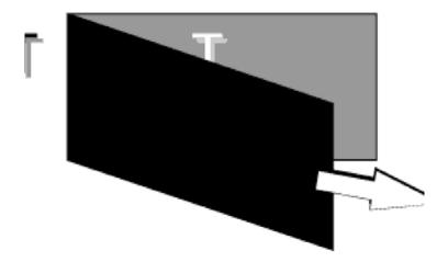
Cautionary Note: Don't wait too long before removal of paper after wetting or delamination of adhesive coating from application tape may occur.
